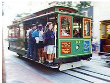
A Cable Car with track & cable trench
