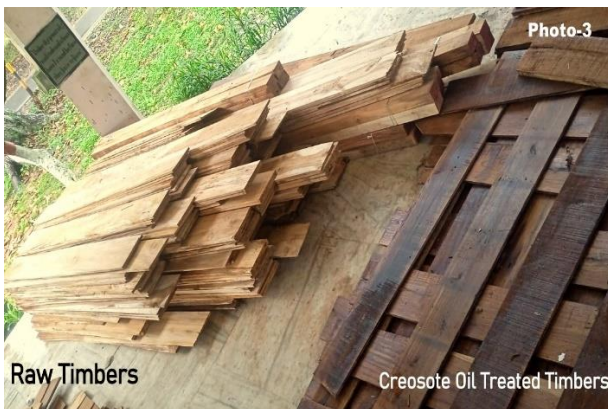
Photo-3 Creosote Oil Treatment of new timbers
